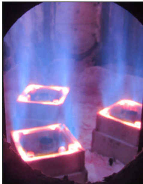
Figure 4: Multi-burner testing of FREE JET Gen 3 burners at Zeeco's Global Technology Center.
